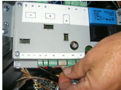
Fig. 2: Plug position on the main board
